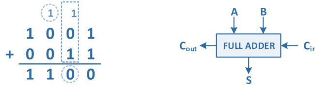
Figure 2.1: Binary Addition and functional block diagram of the one-bit full adder
